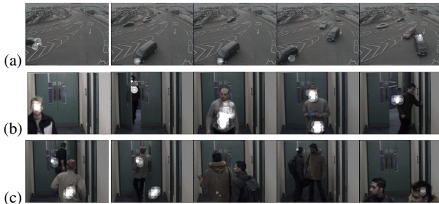
Figure 4: Frames illustrating the ranked top 10% least frequent co-occurrence elements from a busy traffic scene (row(a)), and a corridor and entrance scene (rows (b,c)) using the basic method from Eqn. (7). Co-occurrences at particular spatial locations are highlighted with circles. Sizes of the circles indicate the scale at which the entropy peaks within that local spatio-temporal neighbourhood and their intensity represents the temporal saliency where lighter shades represents higher values.
