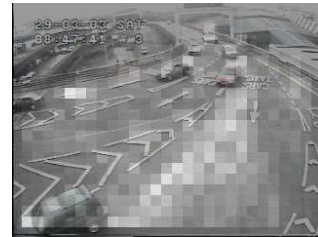
Figure 5: Mean saliency values over time for the traffic scene. Lighter areas show higher saliency. This highlights the problem of biased saliency values due to perspective.
