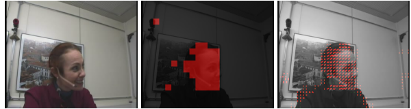
Fig. 2. Compressed-domain video features: From left, original, detected skin-color blocks, motion vectors.
